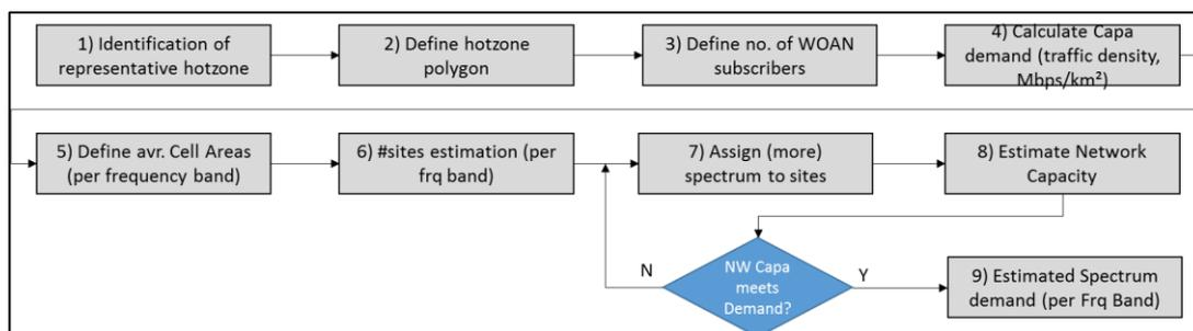
**Figure 1. Best Practice Methodology for Computing Spectrum Requirement**
