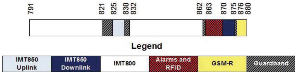
Figure 1: Channel Arrangement for frequency band 825-830 MHz paired with 870-875 MHz
